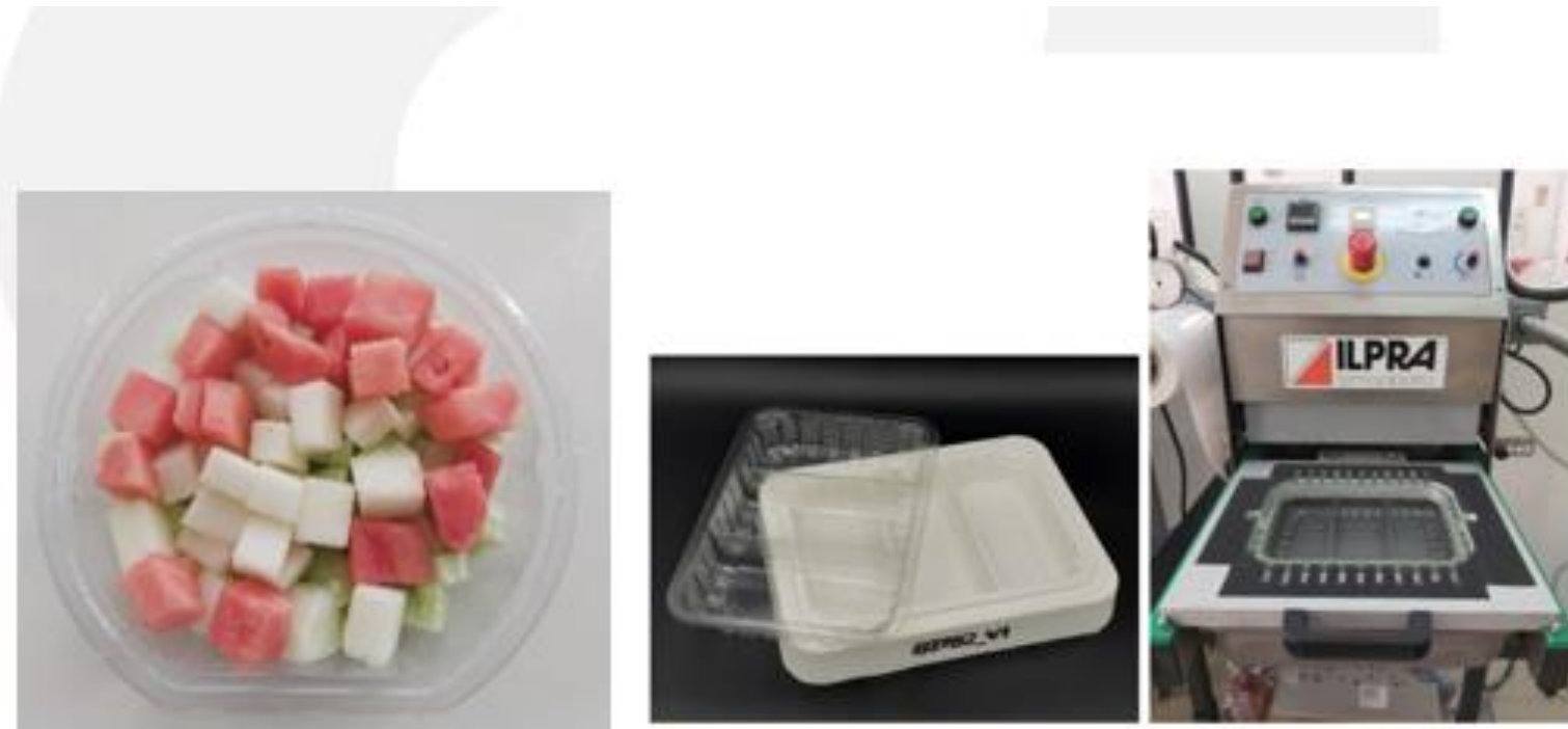
Figure 11: AiNIA tray 3D mold and thermoformed tray on the AiNIA thermoforming equipment.
