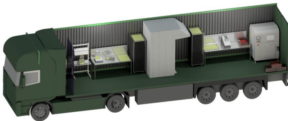
Figure 2. The drying unit including the PEF pre-treatment unit inside the container and all auxiliary devices.
